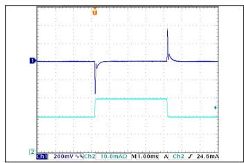
Figure 5: Output voltage response to step-change in load current (50%-75%-50% of lout(max);  $dI/dt = 0.1 \ A/\mu s$ ). Load cap:  $1 \ \mu F$  ceramic and  $15 \ \mu F$  tantalum capacitors. Ch 1: Vout, Ch 2: lout(2.0A/div).
