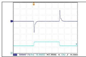
Figure 5: Output voltage response to step-change in load current (50%-75%-50% of lout(max);  $dI/dt = 0.1 \ A/\mu s$ ). Load cap:  $1 \ \mu F$  ceramic capacitor. Ch 1: Vout, Ch 2:  $I = 1.04 \ A/\mu s$ .
