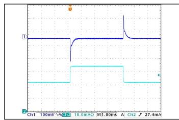
Figure 5: Output voltage response to step-change in load current (50%-75%-50% of Iout(max);  $dI/dt = 0.1 A/\mu s$ ). Load cap:  $1 \mu F$  ceramic and  $15 \mu F$  tantalum capacitors. Ch 1: Vout, Ch 2: Iout(10.0A/div).
