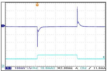
Figure 5: Output voltage response to step-change in load current (50%-75%-50% of lout(max);  $dI/dt = 0.1~A/\mu s$ ). Load cap:  $1~\mu F$  ceramic and 15  $\mu F$  tantalum capacitors. Ch 1: Vout, Ch 2: I = 1.0 t (5.0 A/di v).
