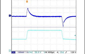
Figure 6: Output voltage response to step-change in input voltage (1V/µs). Load cap: 1 µF ceramic and 15 µF tantalum capacitors. Ch 1: Vout, Ch 2: Vin.
